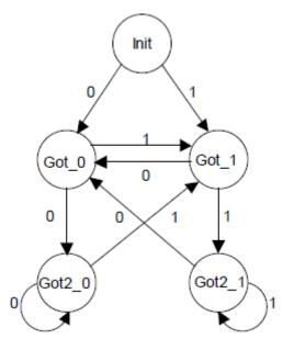
The system starts in the system *Init*. If the input x is 1 on the next clock edge then the system moves into state  $Got_1$ . Similarly, if x is 0 on the next clock edge then the system moves into state  $Got_0$ .
